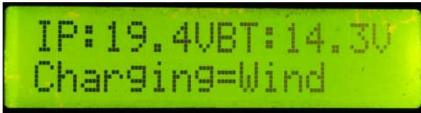
Fig. 7 Message Displayed on LCD When Input Voltage is Above threshold voltage
